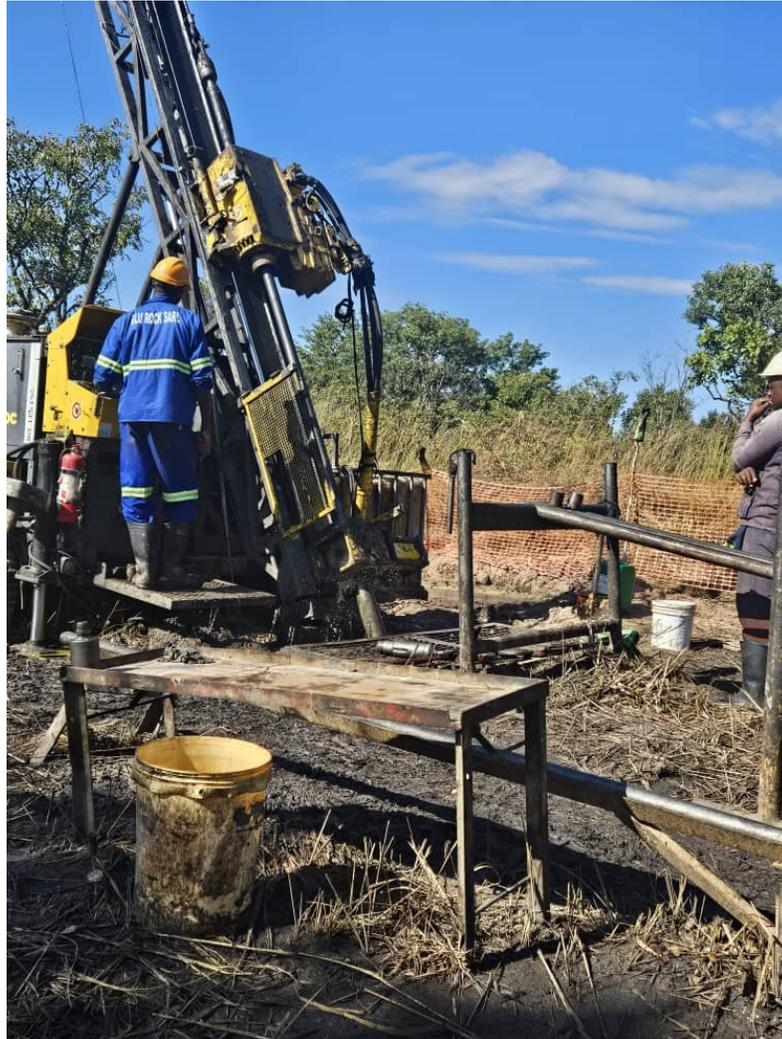
**Figure 43 Machine de forage DD (Diamond drilling)**
